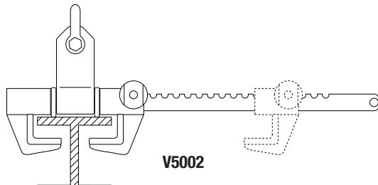
The BeamSlide sliding beam anchor is a mobile device designed for personal fall protection on structural beams. The flange widths range from 4 to 14 in. (100 to 355 mm) and flange thickness up to 1.5 in. (38 mm).
